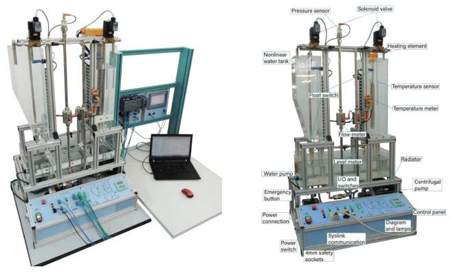
The system includes demo software for basic commissioning, PI level control, PID temperature control, and non-linear control. These features accelerate the learning curve for developing process control PLC programs in a realistic training environment. The BPCLS is an ideal solution for individuals and organizations that want to improve their process control skills and gain a deeper understanding of industrial equipment and processes.
